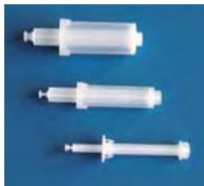
Dispensing cartridges seripettor® 2, 10 and 25 ml
